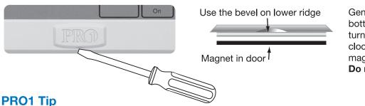
Gently slide a screwdriver into the bottom edge of the badge. Gently turn the screwdriver counter clockwise. The badge is held on by a magnet. The badge should pry off easily. Do not use force.
